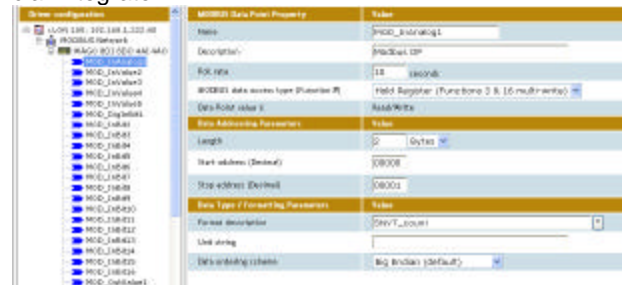
Picture above: "Modbus" Example Wago Analog In.
